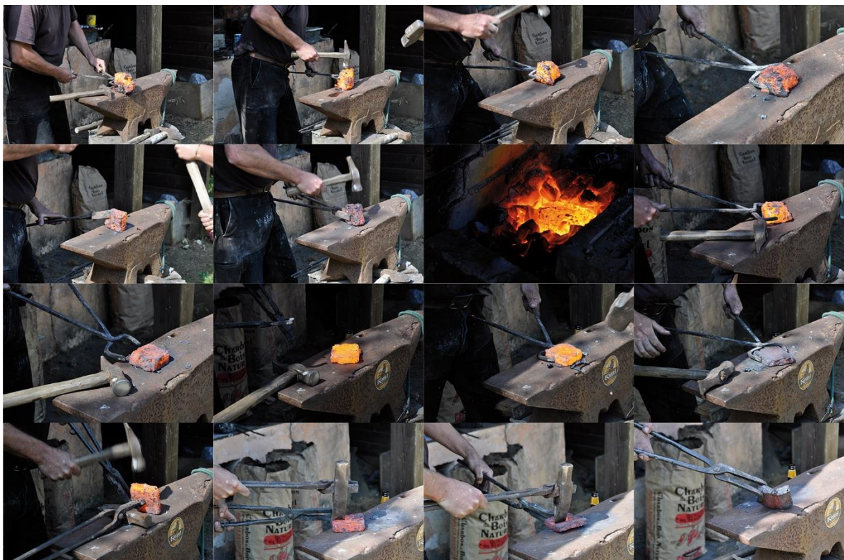
Fig. 1: Sequences 1_1_1 and 1_2_1 of bloom refining and shaping of the two bars (hot cutting of the refining bloom into two bars.). Reading from left to right and top to bottom.
