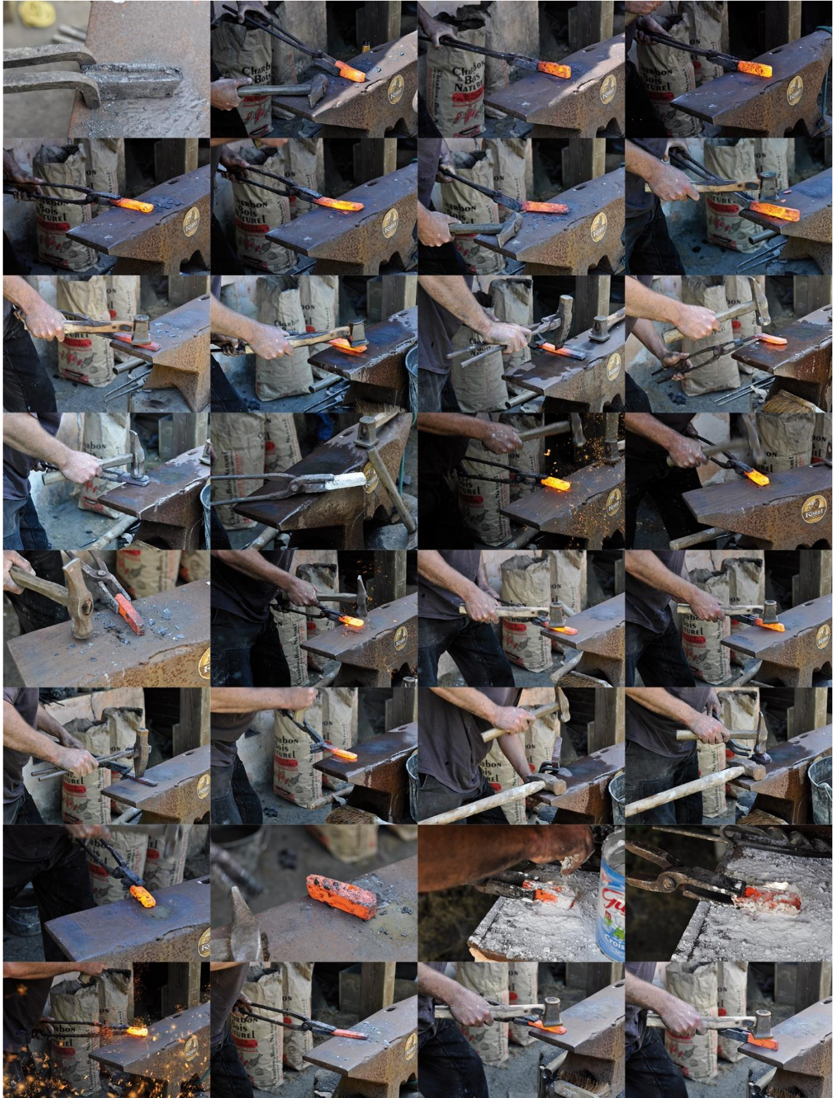
Fig. 2: Sequences 1_1_2 and 1_1_3 of elongating the bar, first folding and welding, elongating the bar and second folding and welding. Reading from left to right and top to bottom.
