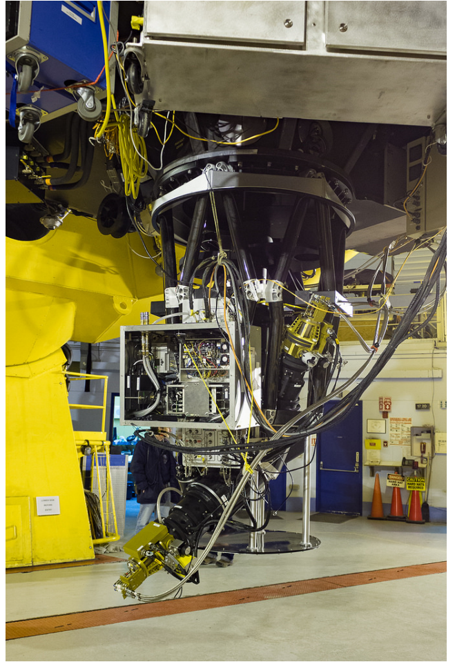
Figure 1. SITELLE at the Cassegrain focus of the Canada-France-Hawaii Telescope (Courtesy Tom Benedict). The two CCD enclosures are in golden color.
