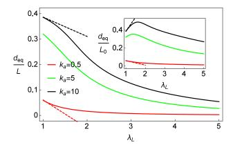
FIG. 9. Deflection of the layer margin as a function of the stretch. The dashed lines are related to the asymptotic formulas (19) (when  $k_a \ll 1$ , red) and (20) (when  $k_a \gg 1$ , black). We show in inset the value of the deflection normalized by the initial length  $L_0$  instead of the actual length. Parameter  $\epsilon_a = -0.4$
