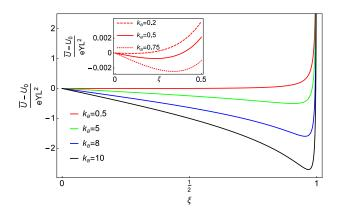
FIG. 5. Dependence of the energy U on the deflection variable  $\xi$  for a given value of  $\epsilon_a = -0.4$ . The inset shows the decay of the energy with  $\xi$  for experimentally relevant values of  $k_a \sim 1$  [29]
