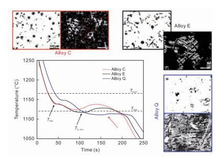
Fig. 1: Experimental cooling curves of the three selected samples (C<sub>uninoc</sub>, E<sub>uninoc</sub>, and Q<sub>uninoc</sub>) and related optical micrographs before and after nital etching. The scale of the micrographs is the same for all and is shown in the upper left one
