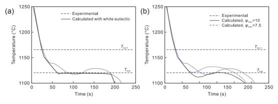
Fig. 3: Comparison of calculated and experimental cooling curves for uninoculated Alloy E: (a) calculation performed accounting for ledeburite formation; (b) calculations performed for two values of  $\varphi_{max}$  and without ledeburite precipitation
