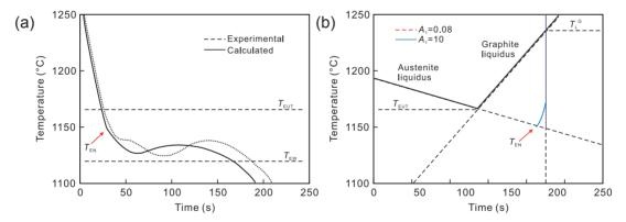
Fig. 2: Comparison of calculated and experimental cooling curves for the uninoculated Alloy C (a), and effect of  $A_1$  value on the solidification path during primary graphite precipitation (b). The red arrow in (a) indicates the slope change associated with appearance of austenite at the calculated  $T_{EN}$  temperature; similarly,  $T_{EN}$  in (b) indicates the corresponding end of primary graphite precipitation when austenite is predicted to appear
