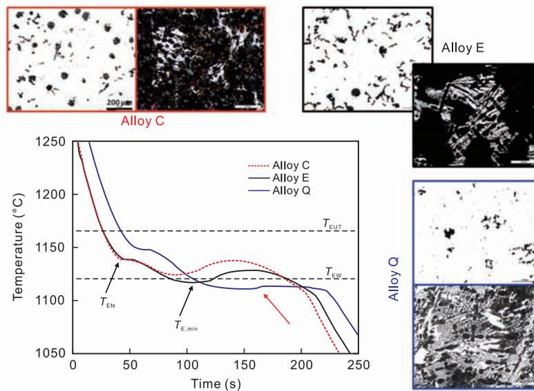
**Fig. 1: Experimental cooling curves of the three selected samples ( $C_{uninoc}$ ,  $E_{uninoc}$  and  $Q_{uninoc}$ ) and related optical micrographs before and after nitral etching. The scale of the micrographs is the same for all and is shown in the upper left one**
