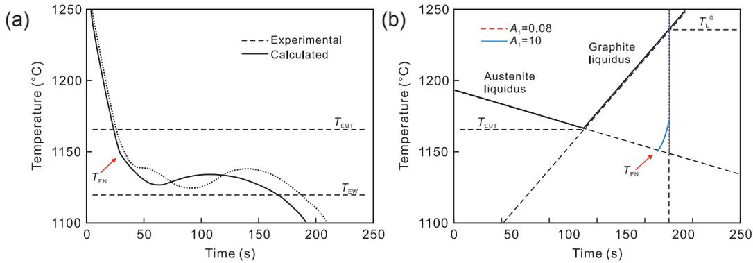
**Fig. 2: Comparison of calculated and experimental cooling curves for the uninoculated Alloy C (a), and effect of  $A_1$  value on the solidification path during primary graphite precipitation (b). The red arrow in (a) indicates the slope change associated with appearance of austenite at the calculated  $T_{\text{EN}}$  temperature; similarly,  $T_{\text{EN}}$  in (b) indicates the corresponding end of primary graphite precipitation when austenite is predicted to appear**
