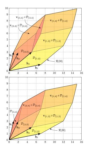
Fig. 1. Partition of  $\mathcal{R}(\mathsf{H})$  into 6 parallelepipeds for two  $2\times 4$  MIMO examples. The example on the top is for  $\mathsf{H}=[7,5,2,1;1,2,2.9,3]$  and the example on the bottom for  $\mathsf{H}=[7,5,2,1;1,3,2.9,3]$ .
