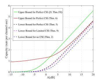
Fig. 2. A  $1 \times 3$  MISO channel, where the entries in  $\mathbb{H}$  follow a Gamma-Gamma distribution, with  $\alpha = 0.4$ .
