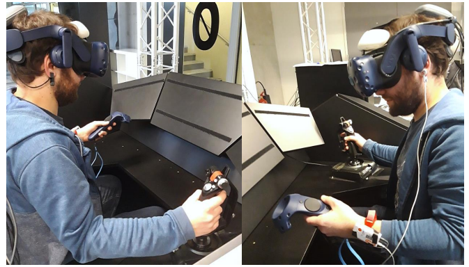
Figure 7: Multiple views of the experimental setup. The user is wearing a Vive Pro Eye equipped with sensors on the headset, a Shimmer3 GSR+ on his left hand, and using a joystick and a Vive Controller on the cockpit.
