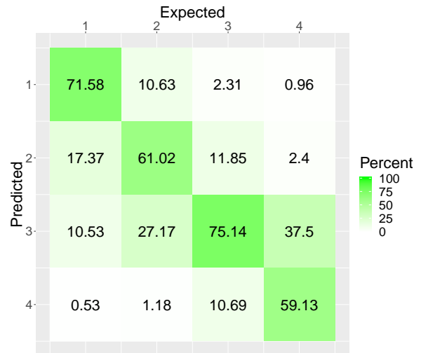
Figure 9: Confusion matrix for “HMD sensors” (Expected and predicted classes) in the “All physio+perf” using NSF normalization setup.
