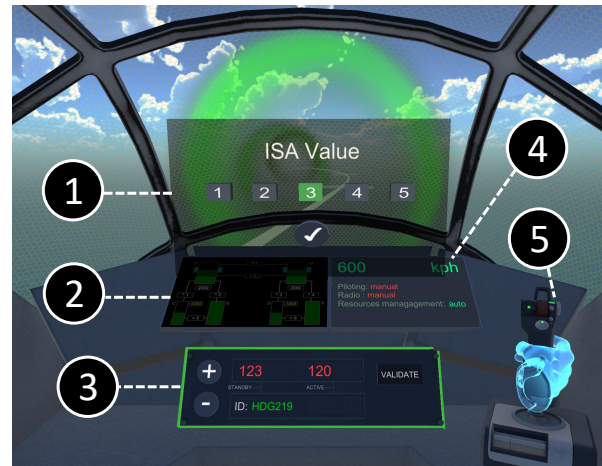
Figure 5: Virtual cockpit view. (1) Instantaneous Self Assessment (ISA) interface. (2) Resources management task interface (deactivated); when activated, the interface lit up (with a green outline). (3) Communication task interface (activated); when deactivated, the interface lit off (no green outline). (4) Informative panel which gives information about which task is activated or not at the current time. (5) Virtual representation of the joystick used to pilot the aircraft and of the right hand. The left hand is represented in the same way, but tracked by a Vive Controller and animated depending on the interaction.
