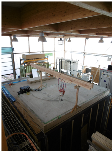
FIGURE 3 – Elastic suspension of the shaker to a wooden beam.
