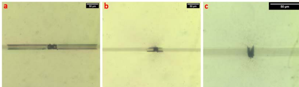
Figure 4: Optical micrographs of the fragmented basalt fibres: (a) as-received, (b) thermally treated and (c) plasma treated basalt fibres.
