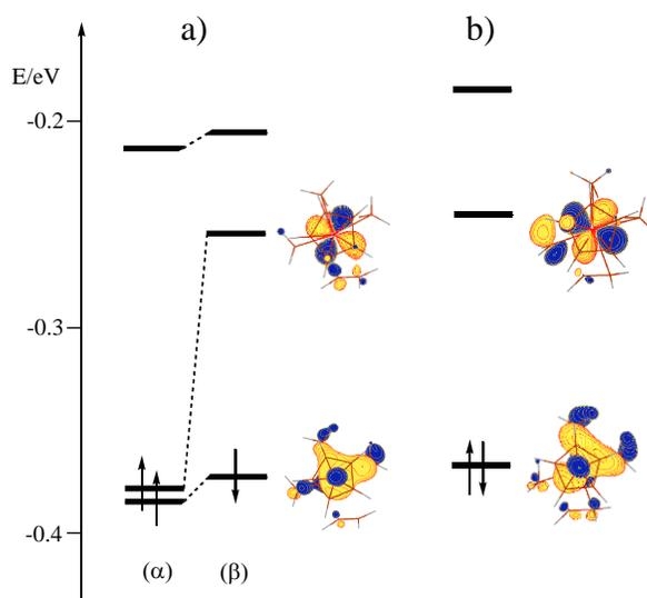
Figure 5. Energy diagram of the Kohn-Sham frontier molecular orbitals for structures  $[\text{CpM}(\text{C}_4\text{H}_6)(\text{C}_2\text{H}_4)(\text{CH}_3)]^+$  (a: M = Mo; b: M = Nb). The contour diagrams shown for the Mo species are those of the  $\beta$  spinorbitals. The corresponding  $\alpha$  spinorbitals have an essentially identical shape.
