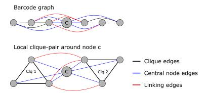
**Figure 1** (Top) linear representation of a barcode graph obtained from 7 molecules of uniform length. (Bottom) The local clique-pair associated to c. In black, the edges from the side cliques of the unit 3-graph. In blue, the edges between the central nodes and the other nodes. In red, the edges between the cliques.
