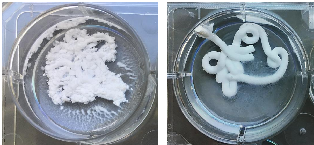
Figure S6. Qualitative assessment of the cohesion of the CPC samples : (a) example of the non-cohesive HBS-0 reference [in 2 wt.% aqueous \text{Na}_2\text{HPO}_4 , extruded 5 minutes after preparation of the paste] showing a disaggregation of the paste after injection in a 0.9 wt% \text{NaCl} solution ; (b) example of a cohesive composite [40/250 CPC composite in 2 wt.% aqueous \text{Na}_2\text{HPO}_4 ,
