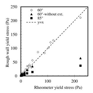
Fig. 12 Influence of the test design on cone yield stress measurement compared to rheometer measurements. The six earths were tested on the  $\beta$ =60° cone, while only REF was tested on the  $\beta$ =85° cone and the cone without extension
