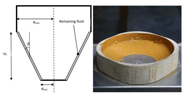
Fig. 5 Left : Cone geometry parameters ; Right : Remaining slip on cone surface after testing
