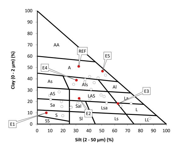
**Fig.1** Clay silt and sand distribution of the 27 collected soil samples. The six red dots correspond to the six samples selected for slip making and rheological studies
