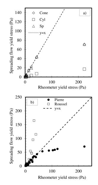
**Fig. 9** a) Yield stress of one slip measured by spreading on sandpaper (Sp) or melamine wood, using a cone or a cylinder (Cyl), using Pierre et al.'s calculus compared with rheometer measurement. b) Yield stress of the six different slips measured by spreading
