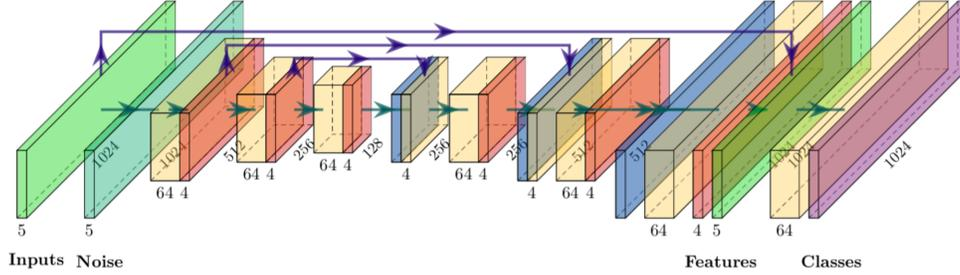
Figure 8: Proposed Network architecture. Yellow boxes represent Conv2D layers of 5x5 with strides (1,2), red boxes Conv2D of 1x1 followed by a dropout of 0.1. Blue color means Upsampling2D layer. Violet arrows illustrate concatenation operator. Note: Original input is directly concatenated to the features computed by the network.
