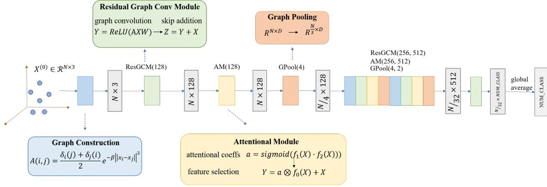
Figure 10: Overall architecture of the proposed Residual Graph Attention Networks (ResGANet). ResGANet consists four main components: graph construction, residual graph module, attention module and graph pooling. The number after ResGCM and ATM denotes the filter number while the number after graph pooling means the pooling stride.
