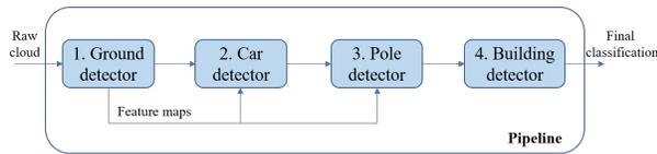
Figure 2: Multi-stage architecture of the vehicle-borne point cloud segmentation process.
