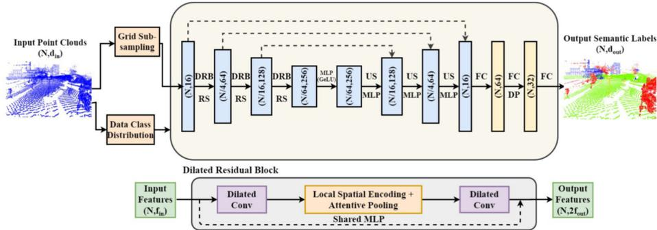
Figure 12: The proposed architecture of GRanD-Net. The abbreviations followed in the architecture are DRB: Dilated residual block, RS: Random sampling, US: Up-sampling, FC: Fully connected layer, DP: Dropout.
