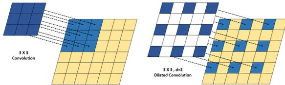
Figure 13: Convolutions: (left)  $3 \times 3$  regular convolution mostly used in CNNs. (right)  $3 \times 3$  dilated convolution with  $d=2$  covering an area of  $5 \times 5$  is used in GRanD-Net resulting in lesser strides and parameters.
