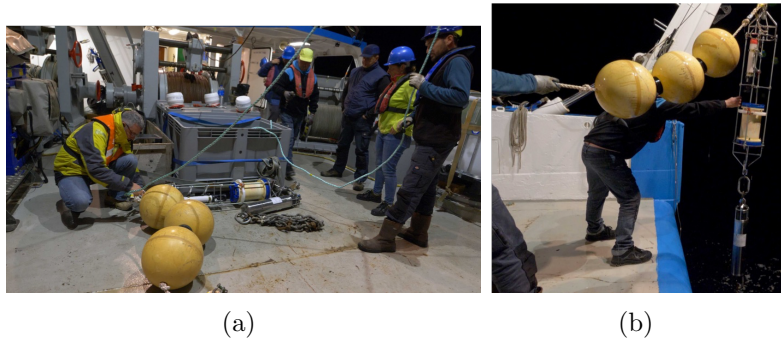
Figure 13: FF-ADCP preparation and deployment. (credit: Hubert Bataille)
