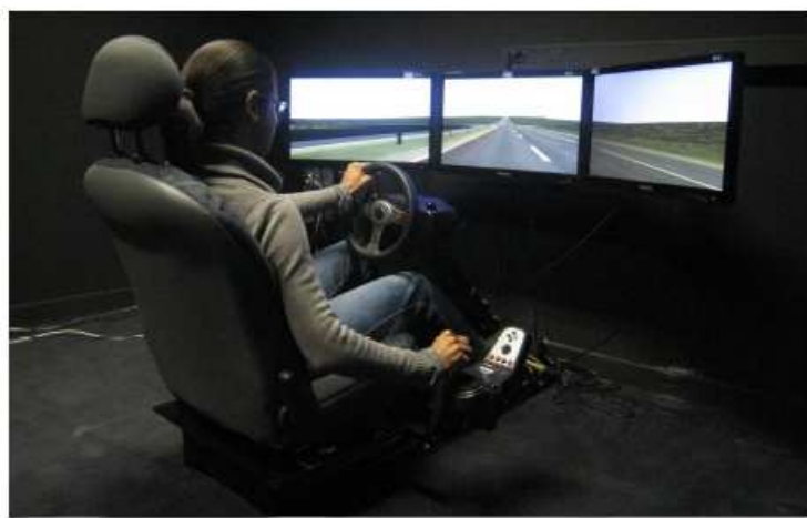
Figure 1. Illustration of the fixed-base driving simulator.
