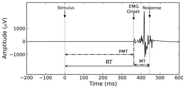
Figure 2. Single-trial RT decomposition using EMG. The Pre-Motor Time  $PMT$  is the time between stimulus and EMG onsets; the Motor Time  $MT$  is the time between the EMG onset and the mechanical response. See Figure A1 for additional examples of EMG recordings.
