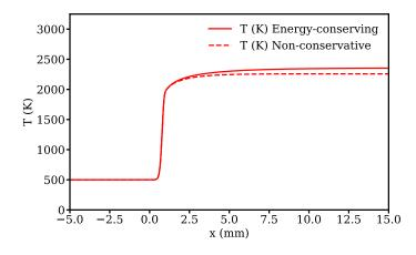
Figure 3. Comparison of the temperature profiles obtained with the energy-conserving model and the nonenergy-conserving one. Same conditions as in Fig. 1.
