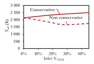
Figure 4. Comparison of the burnt gas adiabatic temperatures obtained with the energy-conserving model (continuous line) and the non-energy-conserving one (dashed line), for varying values of inlet TiCl<sub>4</sub> mass fraction. The fresh gas composition corresponds to  $\phi = 0.8$ .
