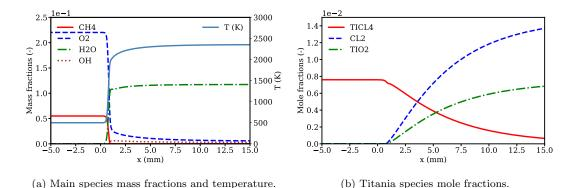
Figure 1. Main species and temperature profiles for the 1D premixed  $CH_4/TiCl_4/O_2/N_2$  flame at stoichiometric conditions. The inlet temperature is 500 K. Injected TiCl<sub>4</sub> mass fraction  $Y_{TiCl_4}^{inj} = 5 \cdot 10^{-2}$ . Results are
