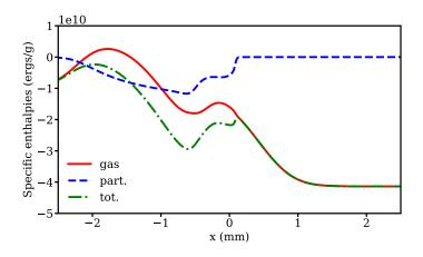
Figure 7. Contributions  $\tilde{h}_{g}$  and  $\tilde{h}_{p}$  of the gas and solid particle phases to the mixture specific enthalpy h. Same conditions as in Fig. 6.
