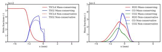
(a) TiCl<sub>4</sub> and TiO<sub>2</sub> mole fraction profiles. (b) M
