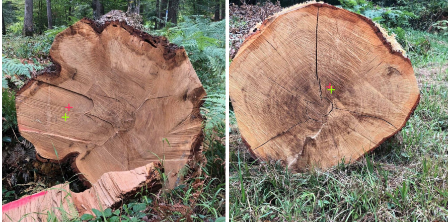
Fig. 13: Examples of wrong pith estimation. Left: The tree rings are in low resolution and the sawing marks are not straight lines. Right: the sawing marks are straight lines but tree rings are in low resolution and really small.
