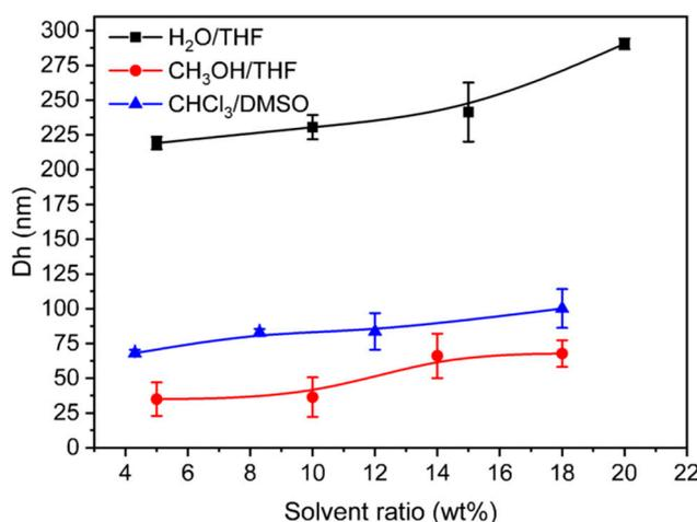
**Figure 6.** Hydrodynamic diameter of the block copolymer brush (sample 1) under selective solvent conditions as measured by dynamic light scattering (DLS). The solvent ratio indicates the proportion of the selective solvent (H<sub>2</sub>O, CH<sub>3</sub>OH, and CHCl<sub>3</sub>).
