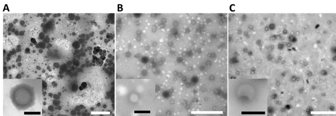
**Figure 7.** Transmission electron microscopy (TEM) pictures of block copolymer brush particles (sample 1) in selective solvent systems. **(A)** THF/water (90/10 *w/w*). **(B)** THF/CH<sub>3</sub>OH (82/18 *w/w*). **(C)** DMSO/CHCl<sub>3</sub> (82/18 *w/w*). Scale bars are all of 1 µm for the main pictures and of 125 nm for the enlargements.
