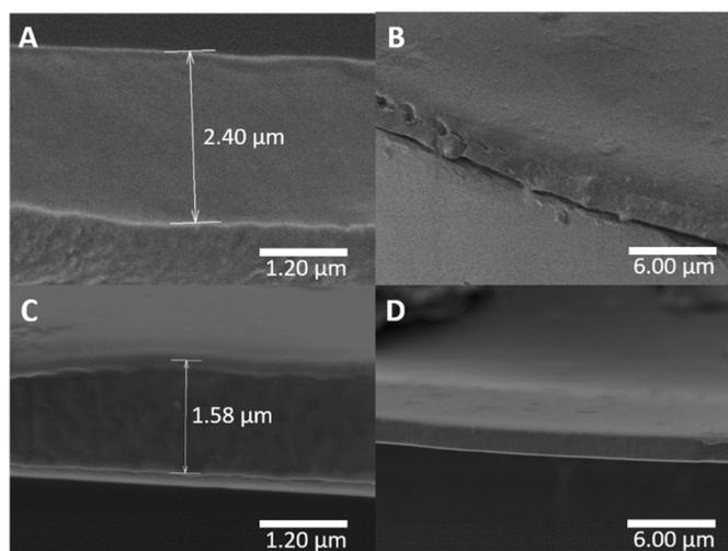
**Figure 8.** Scanning electron microscopy (SEM) pictures (cross section and top view) of the block copolymer brush films made from sample 1. (A) and (B) Film prepared from THF polymer solution. (C) and (D) Film prepared from the THF/water solvent system.
