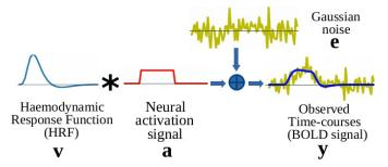
Figure 1: Illustration of the voxelwise BOLD signal modeling:  $\boldsymbol{a}$  is a time series encoding the neural activation signal,  $\boldsymbol{v}$  being the haemodynamic response function (HRF) and  $\boldsymbol{e}$  the additive white Gaussian noise. The measured fMRI signal is denoted  $\boldsymbol{y}$  and obtained via  $\boldsymbol{a}*\boldsymbol{v}+\boldsymbol{e}$ .
