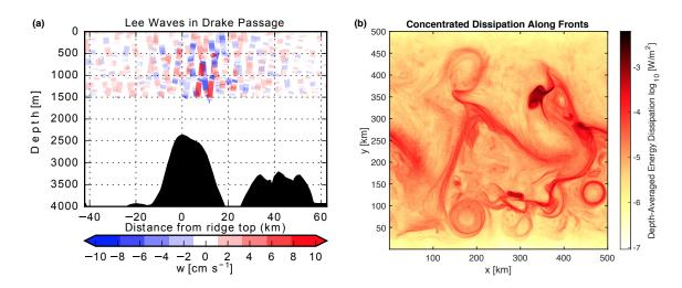
FIGURE 6. Two mechanisms for internal wave generation from geographic current. (a) Vertical velocity associated with lee waves in Drake Passage observed using profiling floats. (b) The vertically integrated energy dissipation in a high-resolution ocean model. Internal waves generated at fronts preferentially dissipate along those fronts. (a) Is from Ref [181] and (b) is modified from Ref [207].
