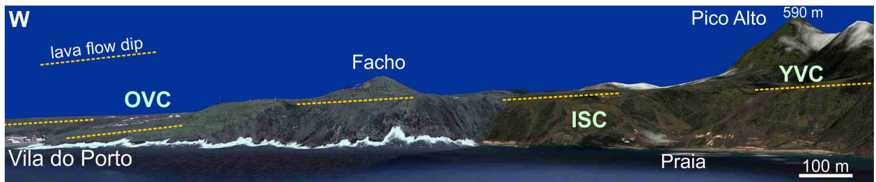
976 Figure S-1. 3-D Google Earth image to show that the gentle slope to the west is mainly 977 structural, i.e. closely follows lava flow dip (dashed orange lines). The steps observed on the 978 topography can therefore represent the front of successive lava flows that did not reach the same 979 distance from the feeder. OVC, ISC and YVC stand for Old Volcanic Complex, Intermediate 980 Sedimentary Complex, and Young Volcanic Complex, respectively. Data from SIO, NOAA, U.S. 981 Navy, NGA, GEBCO.
