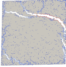
Figure 9: Willam loading: final crack pattern, macroscopic response and evolution of the ratio of broken beams (dashed line).
