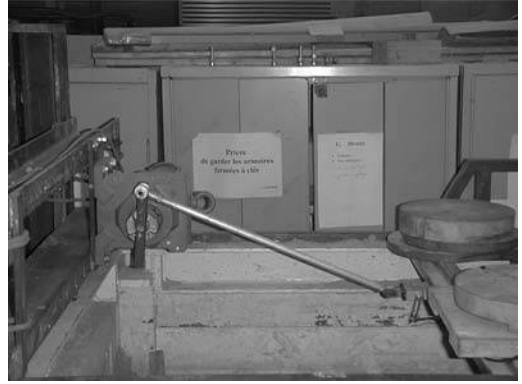
Figure 2. Loading system for displacement controlled tests.
