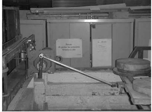
Figure 2. Loading system for displacement controlled tests.
