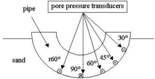
Figure 12. Distribution of the pore pressure sensors along the pipe-soil interface.
