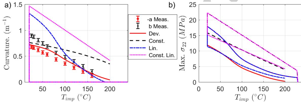
Figure. 13: a) Evolution of the curvatures from the measurement and the four different models b) Estimated evolution of the maximum transversal stress  $\sigma_{22Max}$  at the centre location O from the different models.
