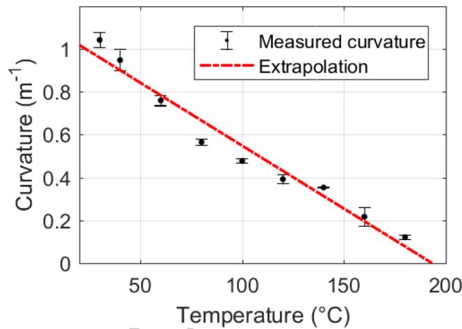
Figure. 4: Evolution of the curvature of [90<sub>4</sub> 0<sub>4</sub>] composite strips to determine the SFT.
