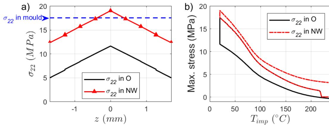
Figure. 11: a) Through-thickness distribution of the stress component transversal to the fibres direction  $\sigma_{22}$  estimated at  $20^\circ\text{C}$  at locations  $O$  and  $NW$ , both in mould and out of the mould b) Evolution of the maximum value of  $\sigma_{22}$  through the thickness of the laminate at locations  $O$  and  $NW$  as a function of the imposed temperature  $T_{imp}$ .
