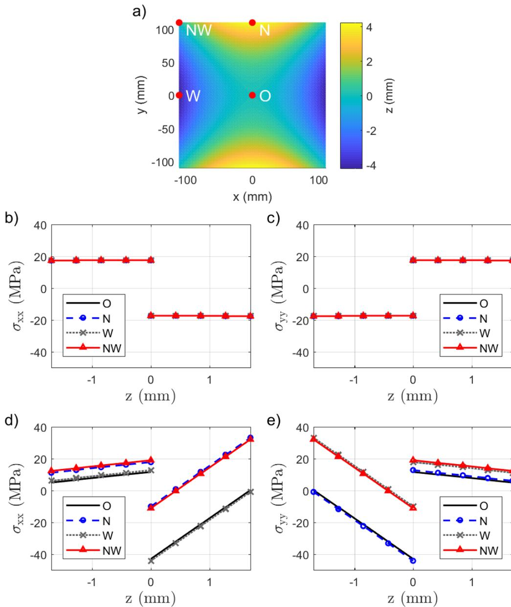
Figure. 10: a) Estimated out of plane displacement  $w$  of the  $[90_4 0_4]$  laminate at  $20^\circ\text{C}$  after demoulding b) and c) Distribution of the in-plane stress component  $\sigma_{xx}$  and  $\sigma_{yy}$ , respectively, at several locations of the laminate before demoulding d) and e) Distribution of the same stress components after demoulding.
