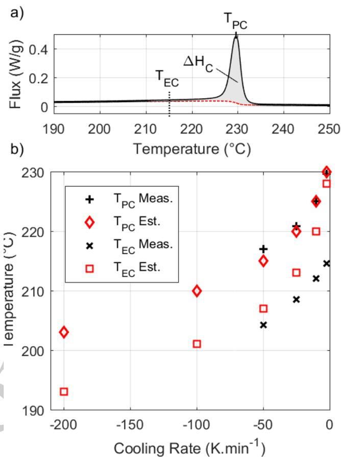
Figure 6: DSC results a) Heat flux obtained during crystallization under a cooling rate of -2K.min<sup>-1</sup> b)
