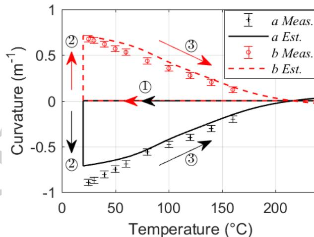
Figure. 9: Evolution of the [90<sub>4</sub> 0<sub>4</sub>] composite plate estimated and measured curvature with temperature. The arrows represent the cooling ①, the demoulding ② and the reheating ③.
