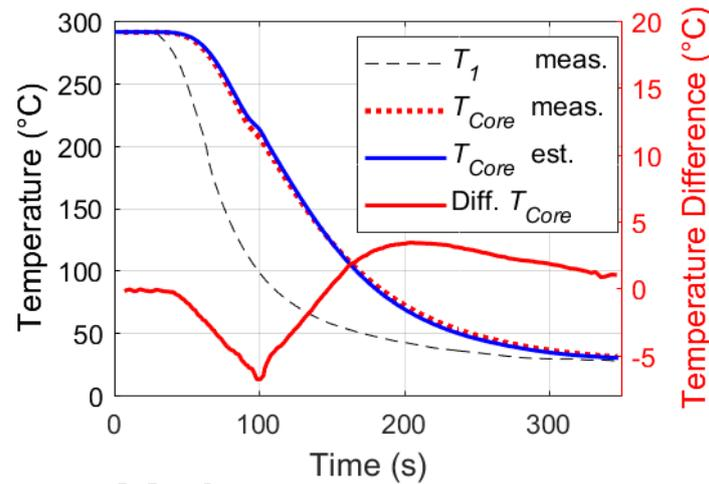
Figure. 8: Measured surface temperature  $T_1$ , measured and estimated core temperature  $T_{Core}$  during the cooling of the composite plate. As a reminder, the maximum recorded cooling rates are of 250 K/min and 130 K/min at the surface and the core of the sample, respectively.
