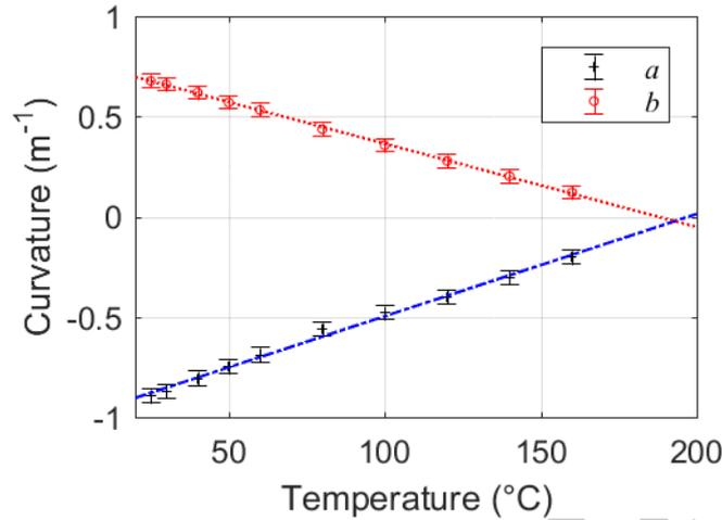
Figure. 5: Evolution of the curvature of the [90\_4 0\_4] composite plates. The markers represent the experimental data and the continuous lines the linear extrapolations.
