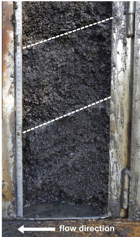
Fig. 8. Photograph of bedload layers visible through the side-wall door of the sampler, showing a ~20° downstream sloping (dashed white lines) deposit.
