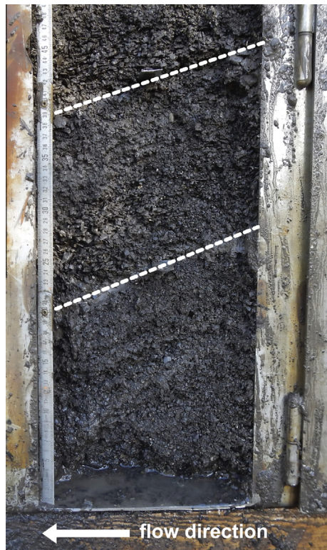
Fig. 8. Photograph of bedload layers visible through the side-wall door of the sampler, showing a \sim 20^\circ downstream sloping (dashed white lines) deposit.
