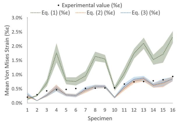
**Figure 2.** Predicted (with an uncertainty of  $\pm 2^\circ$ ) and measured mean von Mises strains for each of non-fractured specimen classified from the smallest experimental measured strain to the largest.
