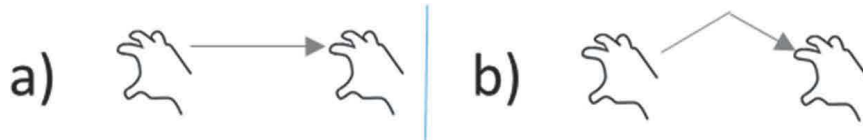
Fig. 1. Tolerance of swipe touch interaction techniques to hardware faults (loss of a line in the hardware grid) – (a) non tolerant (b) tolerant
