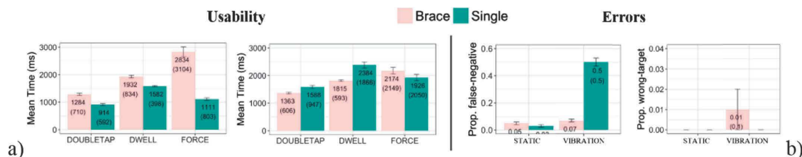
Fig. 8. Target selection times with Braced and Single-Finger selections in static (left) and vibrating (right) conditions [12].
