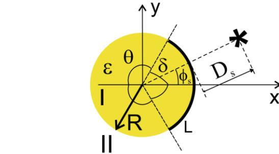
Fig. 1. Cross-section of a dielectric rod with a conformal graphene strip illuminated by a magnetic line current
