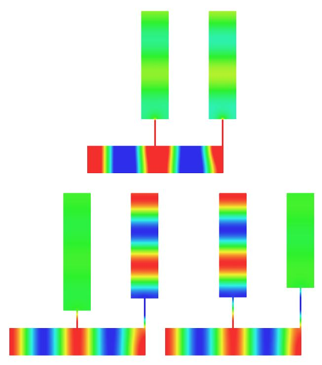
Figure 5: First line: without particular tuning of the lengths of the slits, the energy of the incoming wave is almost completely backscattered. Second line, left: setting where  $R^{\varepsilon}\approx 0$ ,  $T_{+}^{\varepsilon}\approx 0$  and  $|T_{-}^{\varepsilon}|\approx 1$ . Second line, right: setting where  $R^{\varepsilon}\approx 0$ ,  $|T_{+}^{\varepsilon}|\approx 1$  and  $T_{-}^{\varepsilon}\approx 0$ .
