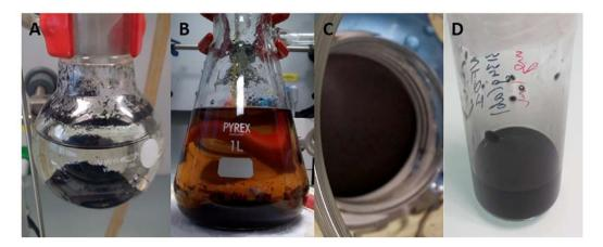
**Fig. 2.** CNF chemical oxidation. A) CNF Solution after cool-down and decantation steps. B) Filtration of the CNF solution on hydrophilic PTFE membrane. C) Picture of the final filtration cake of the PTFE membrane. D) CNFs dispersion at 2 mg/mL concentration in DIW.
