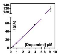
Fig. 6. Linear regression curve of PEDOT-CNF microelectrode current response at 130 mV  $\nu s$  SCE to dopamine injections. The currents steps in the figure correspond to stepped concentrations increase from 0 to 9  $\mu$ M.
