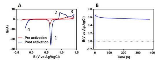
**Fig. 3.** Microelectrode activation. A) CV in  $H_2SO_4$  0.5 M at 200 mV/s between -0.4 and 1.5 V, of a gold microelectrode (20  $\mu$ m diameter) before and after activation (10 cycles of CA at 2 V for 250 ms and 0 V for 1 s). B) Voltammetric response of the microelectrode during deposition under constant current deposition.
