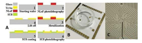
**Fig. 1.** MEA microfabrication. A) MEA microfabrication steps from the starting 4-in. glass wafer to the final SU8-coated wafer. B) Picture of a final functional MEA after glass well gluing. C) Optical picture of the microelectrode matrix.
