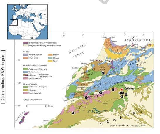
Q10 Figure 1 Moroccan geological structural units and location of the main Pb bearing mines. 1- Jebel Addana, 2- Jebel Aouam, 3- Bou Madine, 4- Imiter, 5- Zgounder, 6- Bou Maiz, 7- Gaouz, 8- Mfis, 9- Tadaout (modified from Frizon de Lamotte et al. 2004). [Colour figure can be viewed at wileyonlinelibrary.com]
