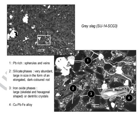
Figure 4 SEM pictures showing the mineralogy of clear and grey slags (Samples SIJ-14-CS6 and SIJ-14-SCG3 respectively).
