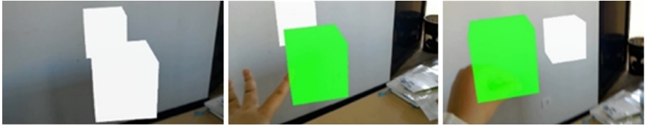
Fig. 12. Select and move a virtual cube with free hand (Color figure online)
