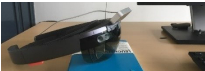
Fig. 1. The LMC is attached on the top of the HoloLens and connected to a computer
