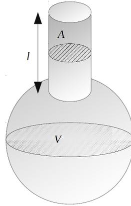
Figure 5. Design of a classic Helmholtz Resonator.
