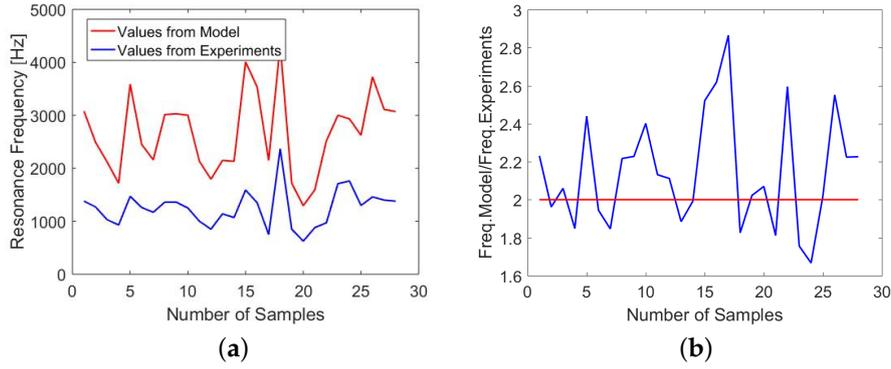
**Figure 9.** Theoretical and measured values of the resonance frequency (a), ratio between both values (b).
