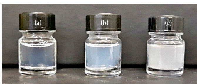
Figure 11. Visual aspects of the micellar solution of the PNVCL- b -PCL (1) block copolymer ( C = 0.5 \text{ mg mL}^{-1} ) at different temperatures, at around: (a) 19 \text{ }^{\circ}\text{C} , (b) 29 \text{ }^{\circ}\text{C} and (c) 40 \text{ }^{\circ}\text{C} .
