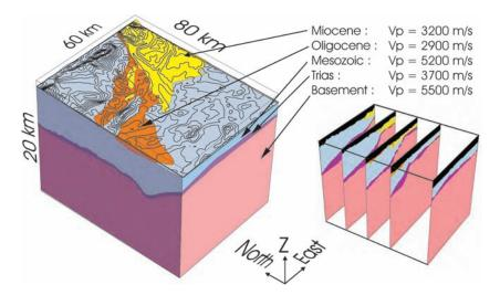
Figure 5: 3-D velocity model with its *P*-wave velocities Vp (Left 3-D numerical bloc where topography is represented by contour lines, right: cross-section views).
