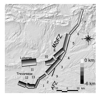
**Figure 4.** Map of simplified MDF segmentation. All segments are numbered, details for each of them are given in Appendix A. Fault plane depth is indicated by a grey scale (from 0 to 6 km depth).
