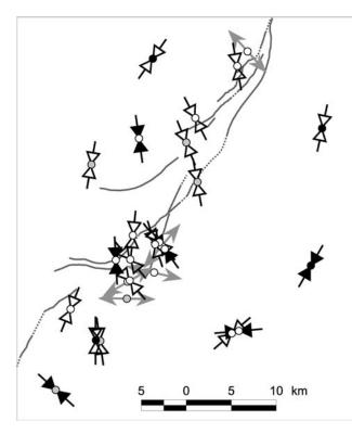
**Figure 8:** *P*- and *T*-axes distribution, deduced from focal solutions (see Fig. 7 for event numbers). Arrow colours indicate different types of faulting mechanisms (black: *P*-axes corresponding to reverse faulting mechanisms; white: *P*-axes corresponding to strike slip mechanisms; grey: *T*-axes of normal faulting mechanisms). Dot colours correspond to absolute depth with respect to sea level (black: below 6 km; grey: between 3 and 6 km and white: shallower than 3 km).
