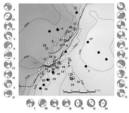
Figure 7. Location map of the 59 best located events around MDF. Circle colours indicate different event depths with respect to basement top (black: events located at least 2 km below basement top; grey: events located less than 2 km above or below basement top; white: events located more than 2 km above basement top. Dashed contours indicate depth of basement top). Focal solutions could be computed for numbered events only, corresponding focal mechanisms are represented around the map.
