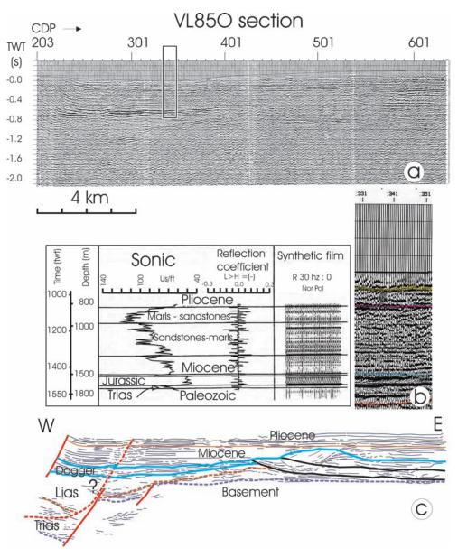
Figure 2. Example of the procedure applied to data used to construct the structural model: (a) Migrated seismic section VL85O, (b) Synthetic film used to identify reflectors and correlation with part of section VL85O (rectangle on Fig. 2a) and (c) Line drawing.
