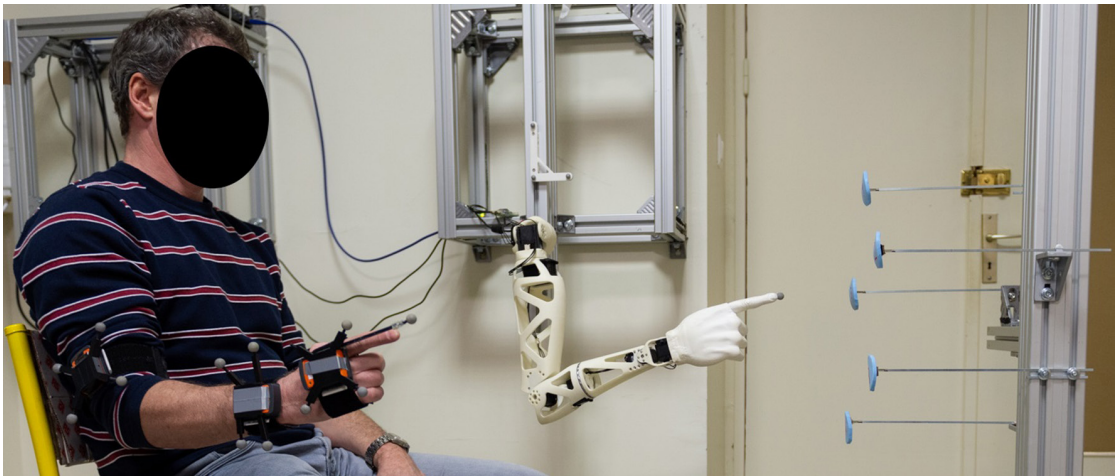
Figure 1. Experimental setup: Both the robot and participant are facing the same way, in front of the targets. Credit © Gautier Dufau.
