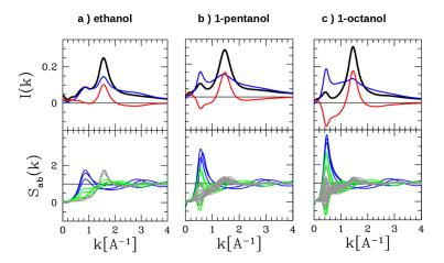
Figure 12: Scattered intensities I(k) (upper panels) and all corresponding atomatom structure factors  $S_{ij}(k)$  for the OPLS model of 3 alcohols (ethanol, 1-pentanol and 1-octanol). The upper panels equally show the like atom contributions to I(k) in blue, and cross atom contributions in red. The lower panels show hydroxyl atom contributions in blue, alkyl tail carbon atom contributions in gray, and cross contributions in green (see text).
