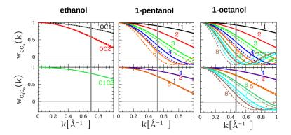
Figure 1:  $w_{XC_1}(k)$  for ethanol, 1-pentanol and 1-octanol, where X=O (upper panels) or X=C<sub>1</sub>(lower panels), and i=1,2,...n. The value of i is shown for 1-pentanol and 1-octanol, next to the corresponding curves. Full curve is with flexibility of alkyl tail and dashed curve without. See text for more details.
