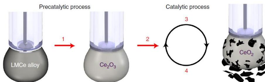
**Figure 5:** Scheme of the CO<sub>2</sub> reduction process constituted by various reactions (1-4), based on Raman measurements. Reproduced from [84], with permission. Copyright 2019, Springer Nature.
