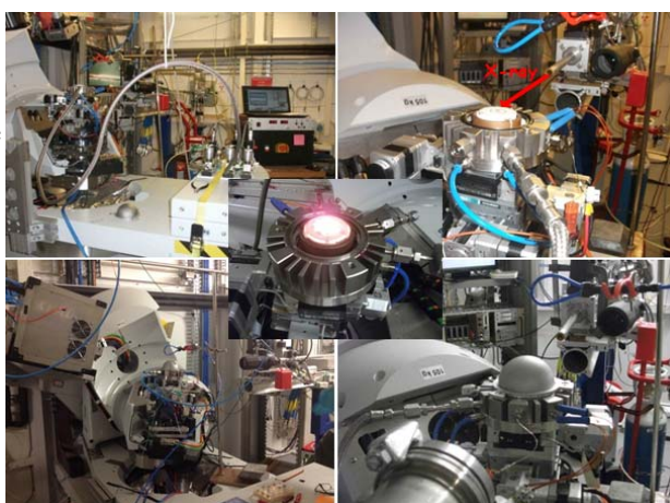
(c) pictures showing the furnace at high temperature on the goniometer and all the associated devices.
