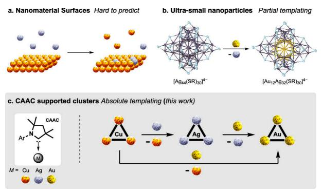
**Figure 1**. (a) Galvanic exchange on a metal surface involving the replacement of a more active metal (orange atom) for a less reducing one (gray atom) is hard to predict. (b) A rare example of multiple atom galvanic exchange in nanoclusters without loss of structural integrity.(11) (c) The stabilization provided by cyclic(alkyl)(amino)carbenes (CAACs) allows for the absolute templating of trinuclear clusters by galvanic exchange.
