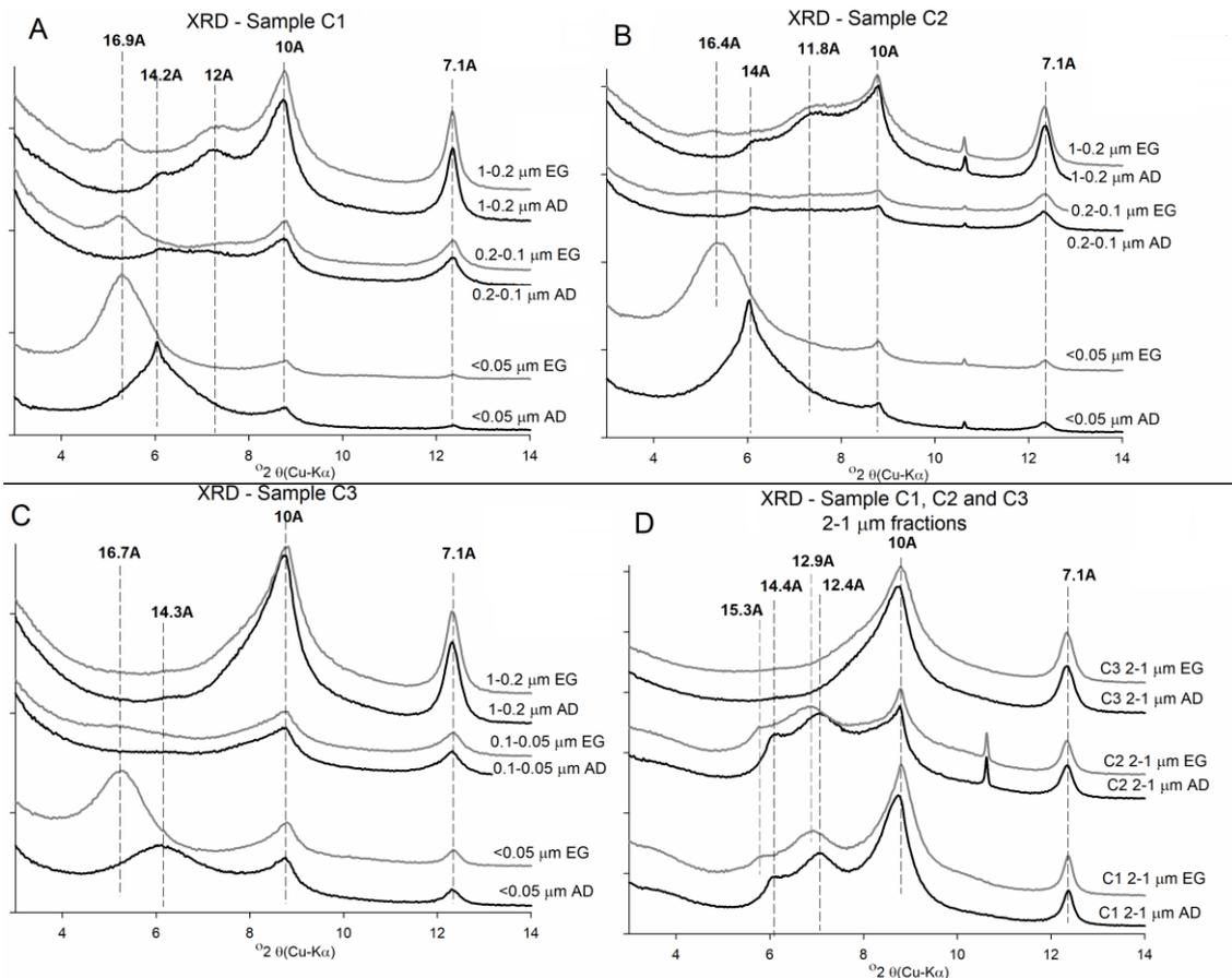
Figure 2 - X-ray diffraction patterns for the three samples C1, C2 and C3 (A, B and C) in air-dried (AD) and after ethylene glycol solvation (EG). Figure D compares the coarse fraction of the three samples
