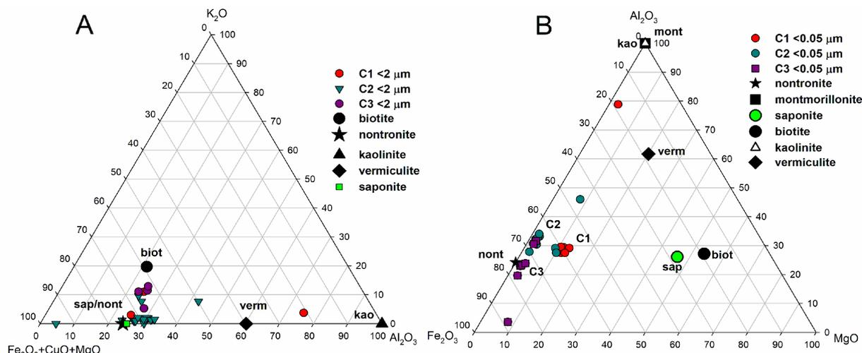
Figure 3 - Ternary diagram for clay mineral particles <2  $\mu\text{m}$  for all samples (A). The theoretical compositions for biotite, nontronite, kaolinite and vermiculite have also been plotted. B - Ternary diagram of <0.05  $\mu\text{m}$  size fraction for all samples. Their composition is close to a Fe-rich dioctahedral smectite (Petit et al., 1992)
