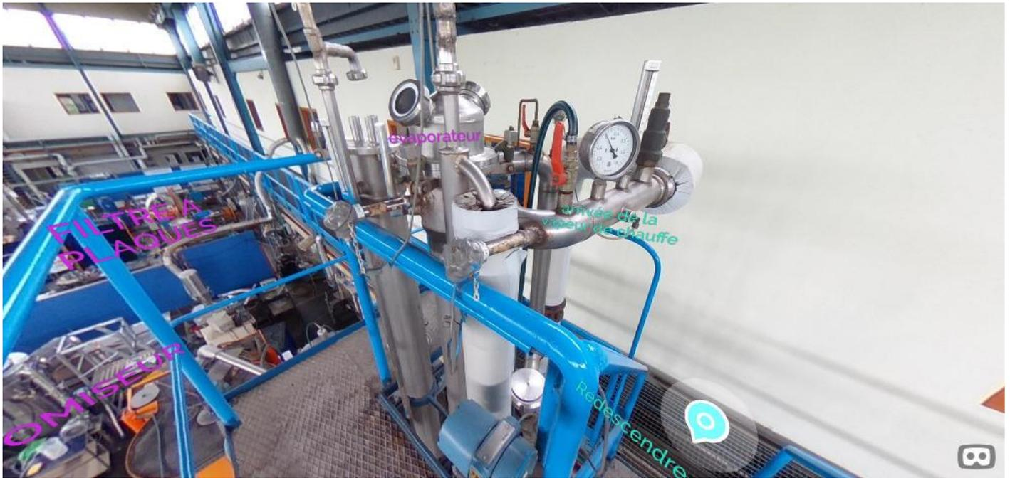
Fig. A7 Example of virtual visit (module #3: falling film evaporator) developed with the online application
