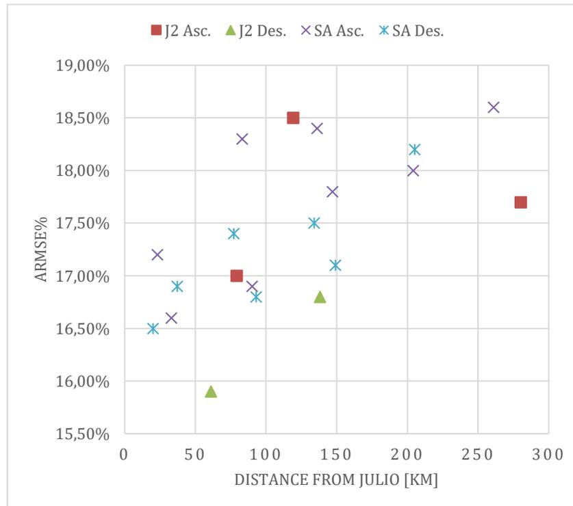
**Figure 3.** Analysis of the sensitivity of the RFA error (in terms of ARMSE%) to the distance from JULIO. Jason 2 and Saral/Altika ARMSE% obtained in the training as function of the distance from JULIO are shown, differentiating the ascending and descending passes.
