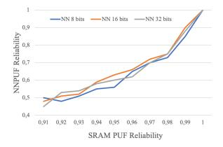
Figure 4: NNPUF Reliability vs SRAM PUF Reliability
